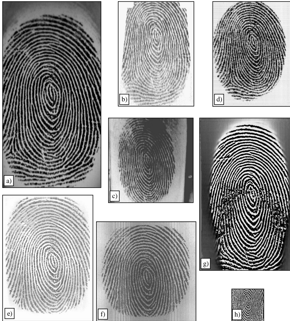
Figure 2.14. Fingerprint images of the same finger with ideal skin condition as acquired by different commercial scanners. Images are reported with right proportions: a) Biometrika FX2000, b) Digital Persona UareU2000, c) Identix DFR200, d) Ethentica TactilSense T-FPM, e) ST-Microelectronics TouchChip TCS1AD, f) Veridicom FPS110, g) Atmel FingerChip AT77C101B, h) Authentec AES4000.
